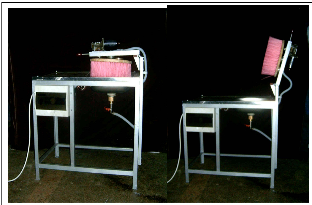
Fig. 9 The cocoon brushing installation in work and open position
